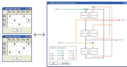
Fig. 3. Dynamic reservation tables and associated pipeline drawn by PipeSim.
