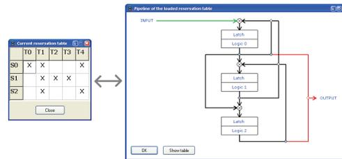
Fig. 2. Static reservation table and associated pipeline drawn by PipeSim.
