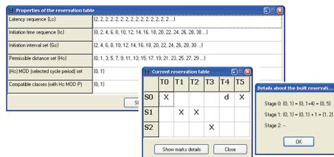
Fig. 7. Example of delay insertion in a static reservation table.
